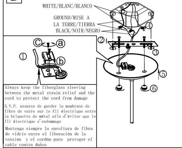
Always keep the fiberglass sleeving between the metal strain relief and the cord to protect the cord from damage
